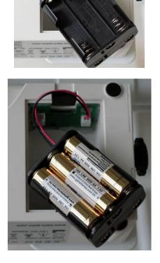
Insert battery holder with the inserted batteries into the display unit
