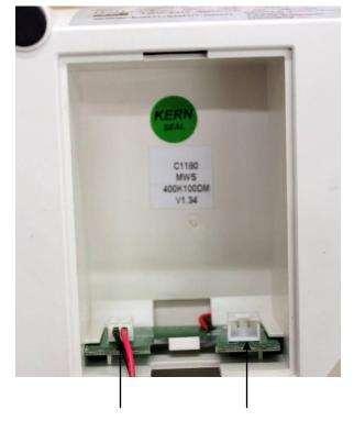
Connection **CN 4** for batteries (AA x 6)
