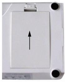
If the batteries are run down, "LO" appears in the display. To turn off, press the  $\overrightarrow{OFF}$  button and immediately change the batteries.
